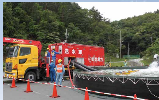
Practice sending water with water truck (backup seawater pump). If the regular seawater pumps cannot be used, the truck pump is used to pump up seawater from the ocean and send it on to the cooling system.
