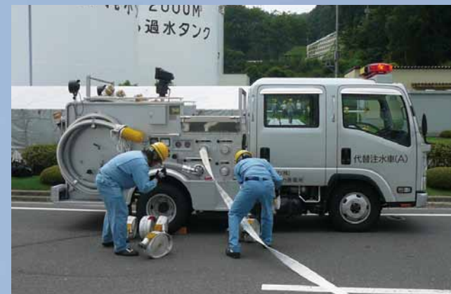
Practice securing water source with backup water truck (portable pump). The water source (condensate storage tank) for supplying water from a tank to a nuclear reactor or spent fuel pool is replenished with coolant.
